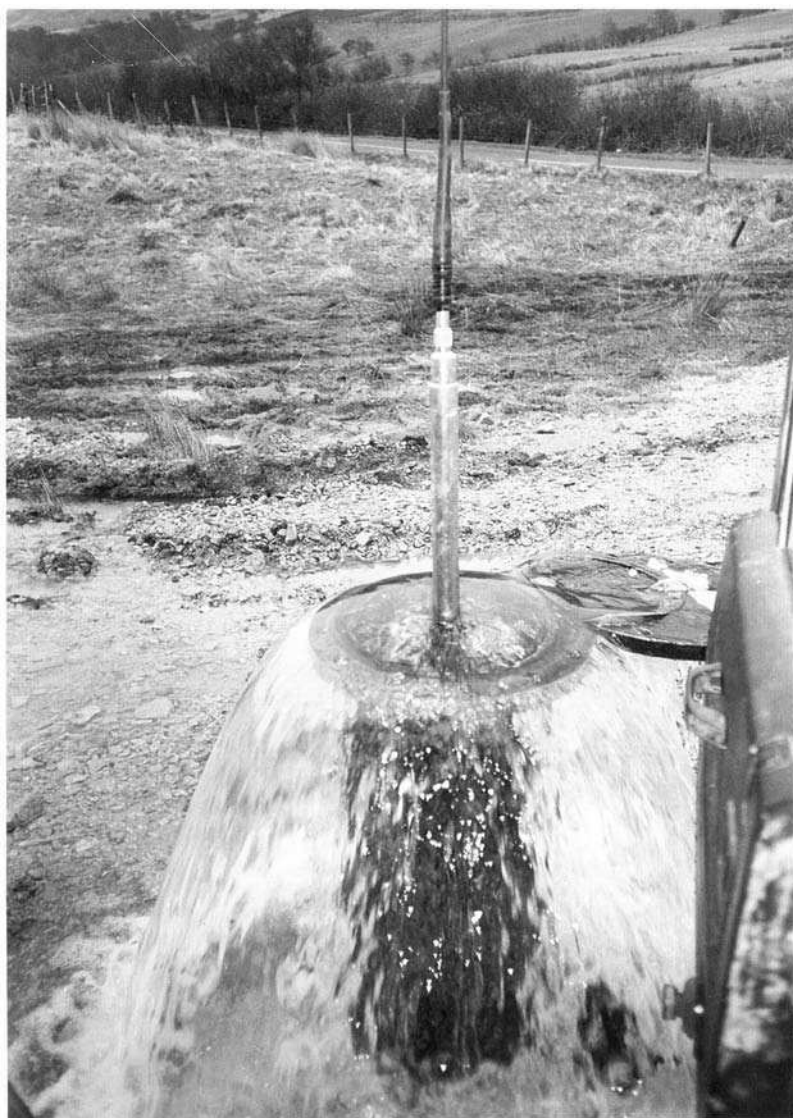
Fig. 2. Geophysical logging of an overflowing borehole in Permian sandstone, Isle of Arran.
